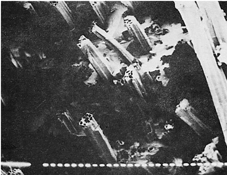
Fig. 7. (200 \times ) SEM of JP composite specimen (dry, no interfacial agent, 40.9% fiber volume) after flexural strength testing, illustrating fiber pullout and damage in addition to transverse fracture.
